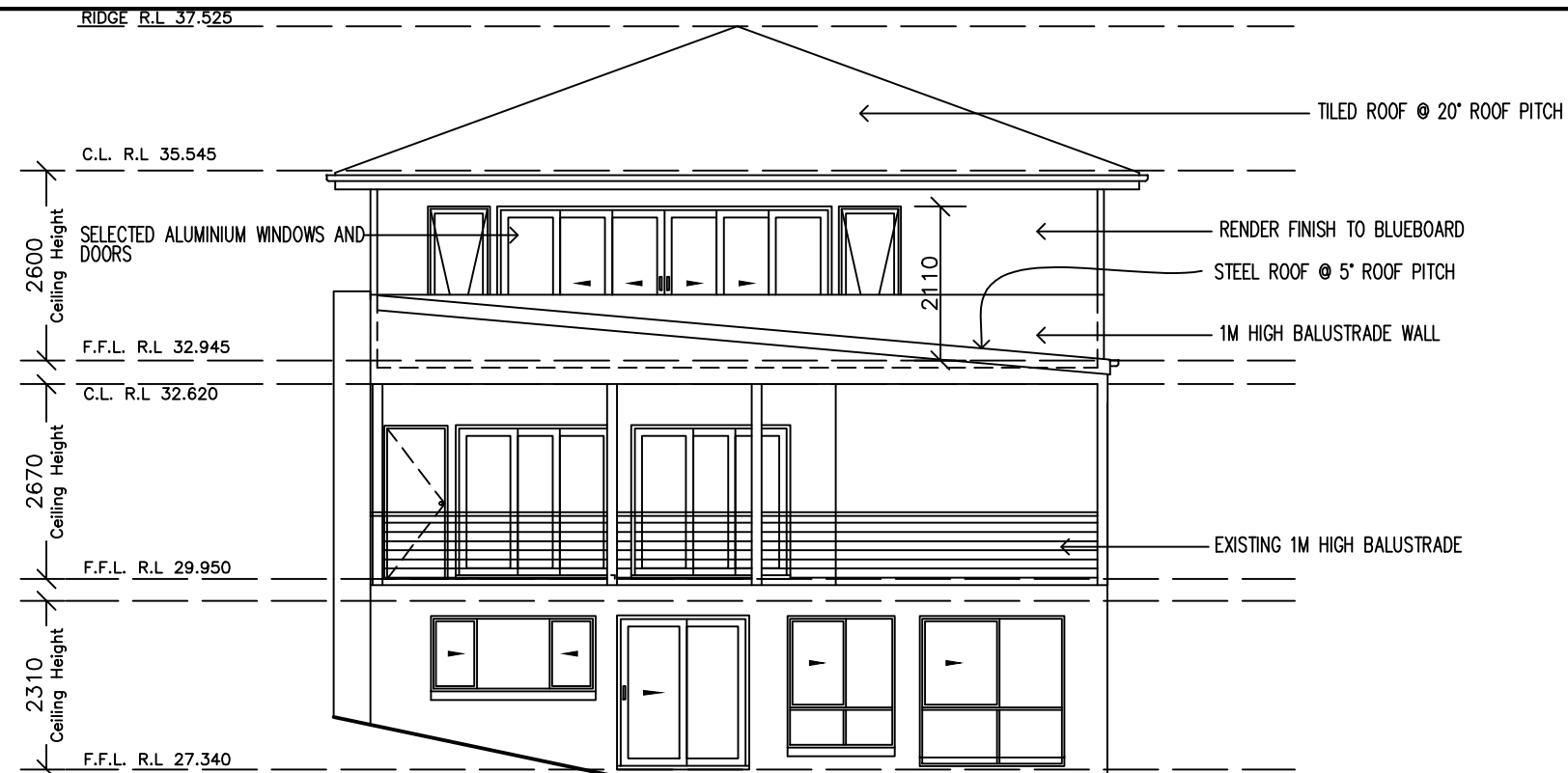
SOUTH WEST ELEVATION
